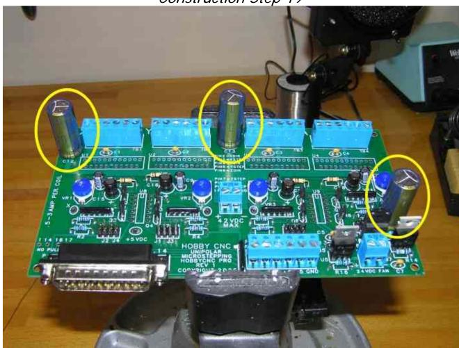
Now we are ready to install the last of the filter capacitors. These three 680uF capacitors go at positions C12, C13 and C14. These capacitors are polarized, which requires them to be orientated correctly when installed on to the board. The longest lead of the capacitor is the positive, which should be inserted in to the hole on the PCB labeled with the "+". The body of the capacitor has a "—" marked on it to assist you in identifying the proper orientation.
