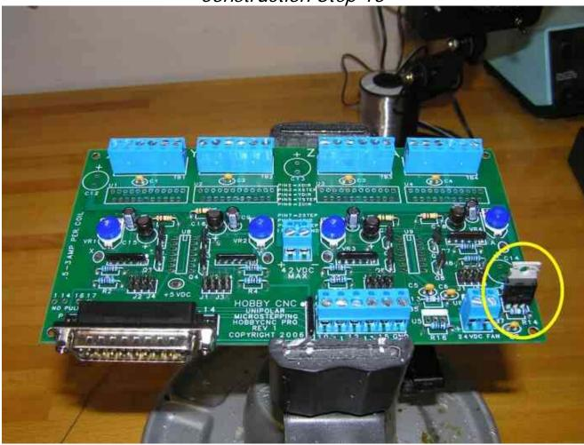
Now we can install the first of three voltage regulators. The first regulator is the LM317HV which goes at position U7. Make sure you install the LM317HV and **NOT the LM317**, which will be installed in a later step. The tab on the back of the regulator should be towards R15. The silkscreen on the board shows the tab as a wide white band.
