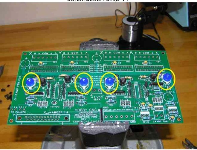
Now we advance to install four variable resistors (potentiometers) at positions VR1, VR2, VR3 and VR4.
