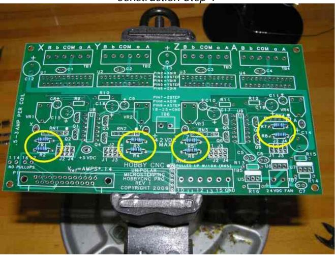
This is where we begin, and you should follow the guide included with the board. The first step is for the installation of eight 10K ohm (Brown-Black-Black-Red-Brown) resistors at location R1, R2, R3, R4, R5, R6, R7 and R8.
