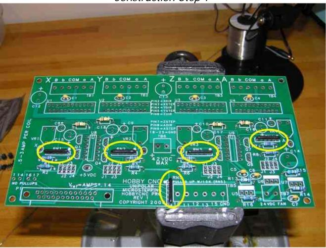
The next step involves the installation of five 10K ohm Resistor Networks at positions RN1, RN2, RN3, RN4 and RN5. Resistor Networks **must** be installed in the correction direction. You should match up the dot on the resistor network with the corresponding dot on the PC board.
