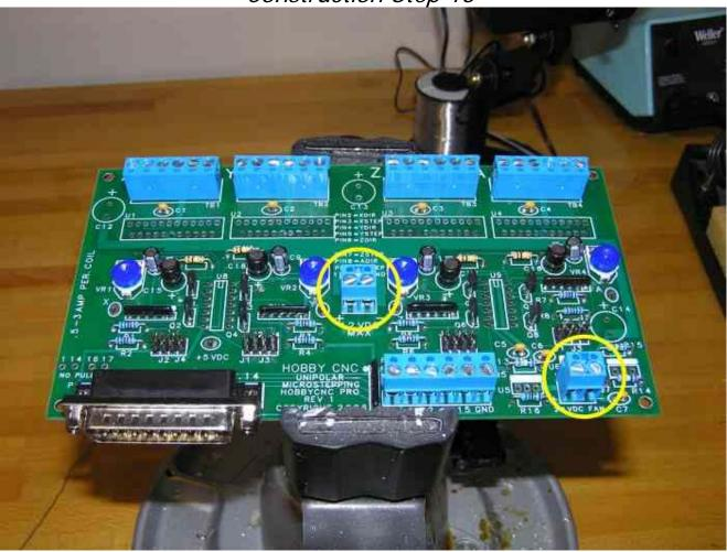
Now install the two smaller two-position Terminal Blocks at TB6, and TB7. Again, these should be positioned with the holes facing the outside edge of the PC board.
