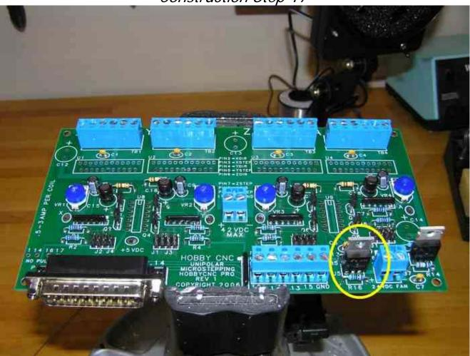
Now install the second of three voltage regulators. This regulator is the LM317 which goes at position U5. The tab on the back of the regulator should be towards R13. The silkscreen on the board shows the tab as a wide white band.
