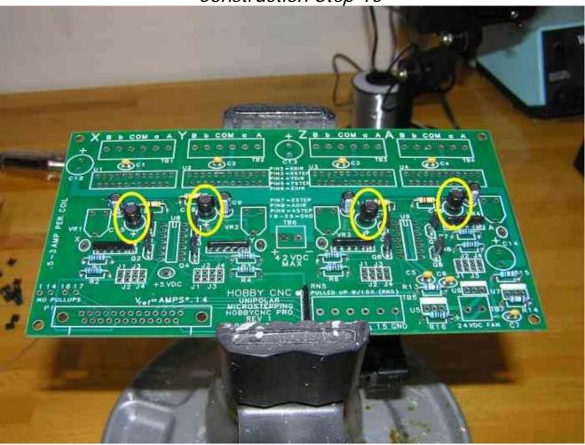
We now move on to four 100uF 16v electrolytic capacitors located at positions C15, C16, C17 and C18. These capacitors are polarized, which requires them to be orientated correctly when installed on to the board. The longest lead of the capacitor is the positive, which should be inserted in to the hole on the PCB labeled with the "+". The body of the capacitor has a "—" marked on it to assist you in identifying the proper orientation.
