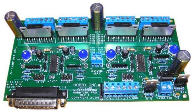
The HobbyCNC PRO Chopper Driver board is one of the more popular stepper controller boards for the hobby CNC market. Good for use on routers, lathes, mills, PCB drillers, engravers — the possibilities are endless.
