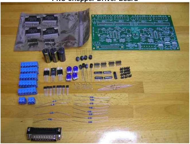
Your first job is to carefully remove all the parts from the package and sort them out. In our kit, we were missing a single .1uF capacitor. Good thing we have a well-stocked parts kit.
