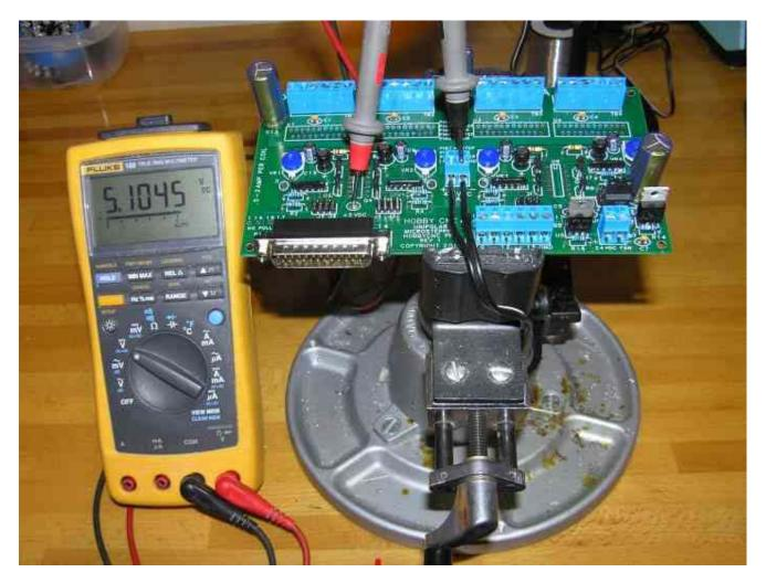
Now we need to verify that the 5v regulator circuit is functioning as intended. The 5v circuit provides power to all the semiconductors on the board, so it is important we have the correct voltage here before installing any of the driver chips.
