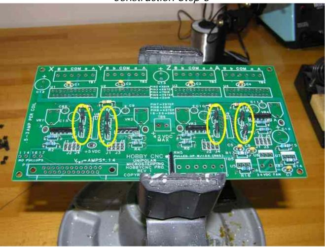
Now it is time to install the Mosfets. Eight of these three-legged devices are installed at positions Q1, Q2, Q3, Q4, Q5, Q6, Q7 and Q8. Care again must be observed when installing these as their orientation must be correct. You will notice that one side of the Mosfet has a round edge, this round edge must match the rounding of silk screen on the PC board. Double and triple check to ensure these are all orientated correctly.
