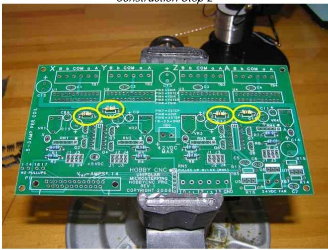
Now we move on to the installation of four 100K ohm (Brown-Black-Yellow-Gold) resistors at locations R9, R10, R11 and R12.
