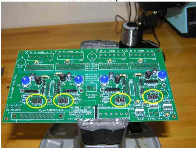
We can now install the header pins at J1, J2, J3 and J4. You can install the jumpers on the header pins prior to installing on the board to allow you to hold on to the pins as you solder them in. Once installed, you should refer to the PCB Connections drawing included with the board which describes the various setting options in more detail.
