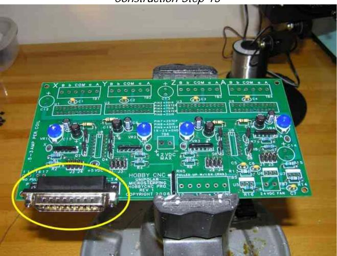
The largest connector on the board is now ready for installation. The DB25 male connector can be installed at P1. Take your time fitting this on to the board as you do not want to damage any of the pins.
