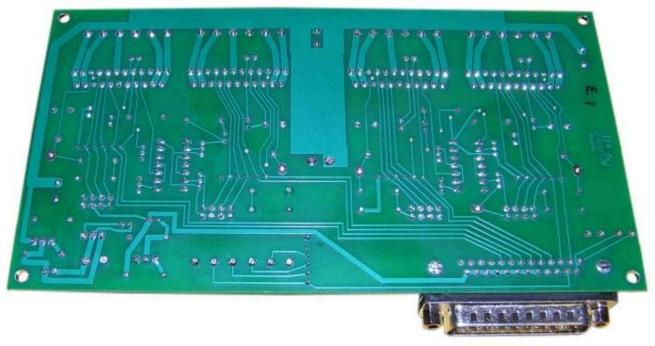
The final step is one of the most important. Clean the PC board with an alcohol or flux remover, or if you used a solder with a water soluble flux, warm water. Carefully inspect all solder connections with a magnifying glass looking for solder bridges or cold solder joints. This step will eliminate almost all possibilities of initial board failures.
