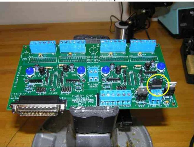
The final regulator, 7824, can now be installation at position U6. The tab on the back of the regulator should be towards C6. The silkscreen on the board shows the tab as a wide white band.
