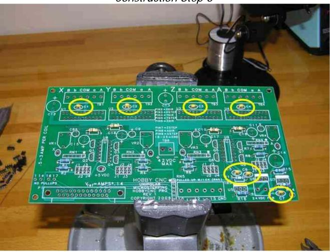
Now we move on to the installation of seven .1uF capacitors at locations C1, C2, C3, C4, C5, C6 and C7. Like resistors, these capacitors have no polarity or orientation – they too can be installed in any direction.
