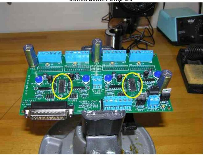
This is where we begin to install the first driver related components. Install two MM74HC14N chips at positions U8 and U9. Be sure to match the pin-1 notch on the chip with the pin-1 notch shown on the PCB silkscreen.
