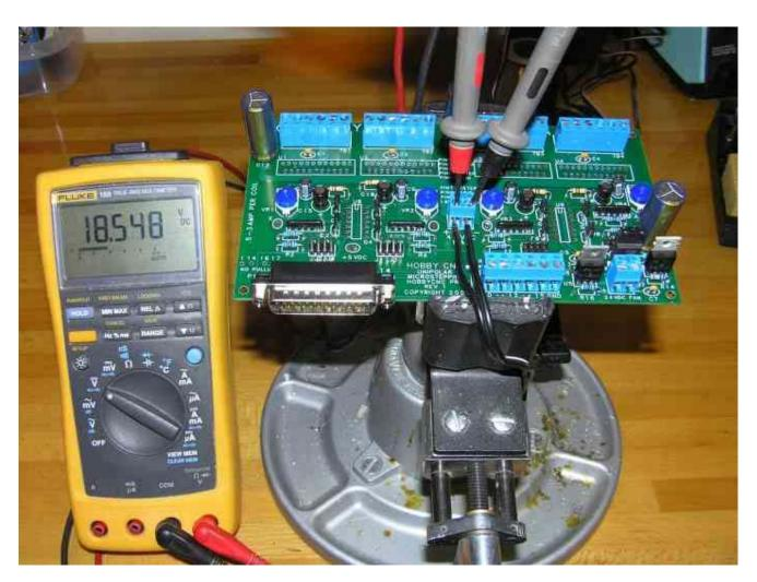
After applying 12v to 42v DC at TB6, you should verify the voltage across TB6 with a volt meter. The black lead of your meter should go to the " –" terminal and the red lead to the "+". In our test case, we have 18.548v being applied to the board.
