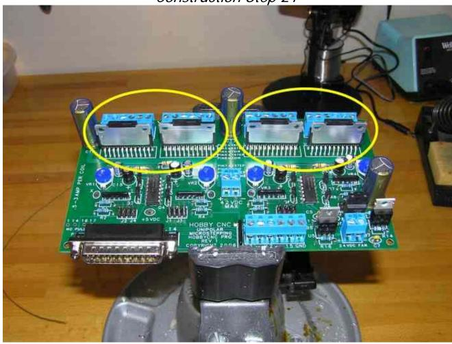
Now we move on to the last components, the driver chips. The four drivers go at positions U1, U2, U3 and U4. With the pin layout on the chips, they can only be installed to the board in one direction. Carefully install each chip ensuring that each pin is inserted correctly into the PCB.
