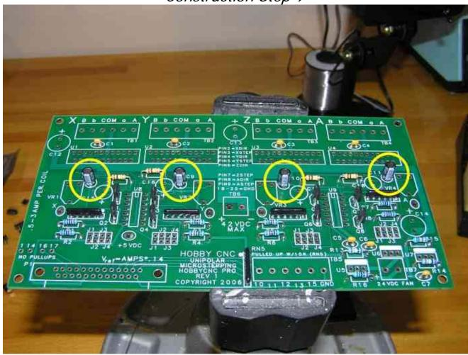
We now move on to four 10uF 50v electrolytic capacitors located at positions C8, C9, C10 and C11. These capacitors are polarized, which requires them to be orientated correctly when installed on to the board. The longest lead of the capacitor is the positive, which should be inserted in to the hole on the PCB labeled with the "+". The body of the capacitor has a "—" marked on it to assist you in identifying the proper orientation. **Do not confuse with positions C15-C18**.
