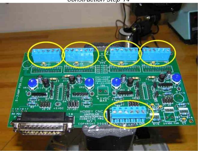
Now install the five large six-position Terminal Blocks at TB1, TB2, TB3, TB4, and TB5. These should be positioned with the holes facing the outside edge of the PC board.
